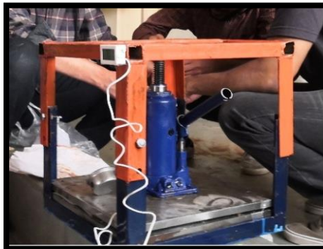
Figure 2. Self-Made compression moulding set-up
